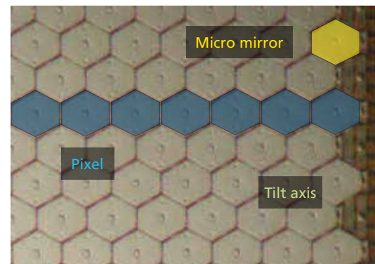
Layout of part of a 1D light modulator.
